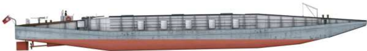
Figure 4: Marinefaehrprahm Type A (Marco Guerik, 2021). Marinefaehrprahm Type D Although the Type A F-lighter was very successfully fulfilling its tasks, improvements were continuously incorporated from war experience up to the new series production designated as Type D. This had better longitudinal strength, a more suitable hull form for navigation, a larger cargo space, a stronger ramp, improved armament, and better crew accommodation. Design work had already begun in 1942. The hull was welded. The reinforced cargo space floor was designed to accommodate heavy loads, such as the 65-ton Tiger tank or a heavy howitzer with a 5.5-ton axle load. The loading space profile corresponded to the railway loading gauge, so all standard cargo and vehicles could be transported.
